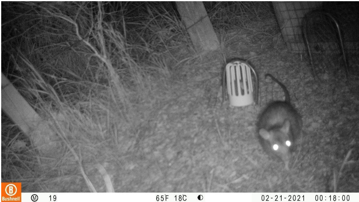
Figure 14: The original camera setup included bait inside the white plastic egg cover used in the trapinator stoat traps.
